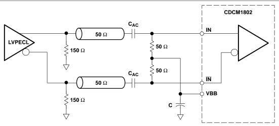
Figure 13. Recommended AC-Coupling LVPECL Receiver Input Termination
