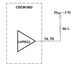
Figure 11. LVPECL Output Loading During Device Test
