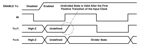
Figure 17. Signal State After an Output Driver Becomes Enabled While IN = 0
