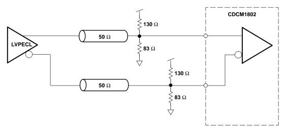
Figure 14. Recommended DC-Coupling LVPECL Receiver Input Termination
