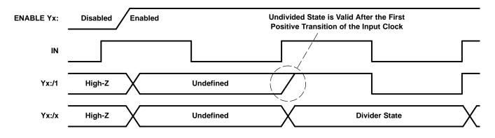
Figure 18. Signal State After an Output Driver Becomes Enabled While IN = 1
