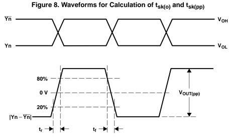
Figure 9. LVPECL Differential Output Voltage and Rise/Fall Time
