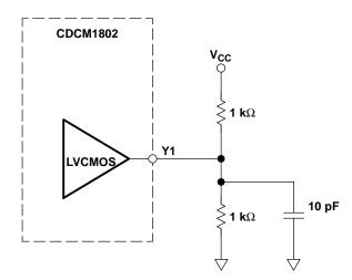
Figure 10. LVCMOS Output Loading During Device Test
